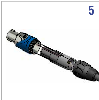
Orientate the insert and cable clamp as shown then push all together into the shell.
