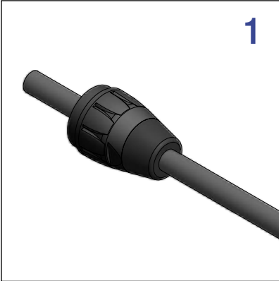
Slide the nut onto the cable
