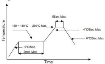
Note: Reflow soldering can be operated only one time. During the temperature ramp-up, no forces may be exerted on the VP which could deform or damage them. After soldering completed, please also do not process until the product temperature ramp down to room temperature.
