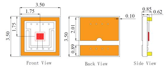
VD-0850I-005W-1D-2A0 with Substrate 1=AIN and Package D=5050 (unit: mm)
