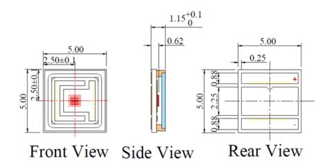
VD-0850I-006W-1F-2A0 with Substrate 1=AIN and Package F=6868 (unit: mm)
