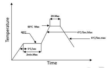
Note: In the PCB baking process, the PCB with VCSEL diode is placed in an oven set at a temperature of 40°C to 60°C at a maximum of 2 hours. It is critical not to overheat the board or bake it for an extended period, as this can cause damage. After baking, it needs to be placed at ambient temperature for 3-4 hours. The test can be carried out after the flux in the silver glue is fully volatilized and an effective metal layer is formed.
