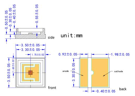
VD-0850I-004W-1D-2A0 with Substrate 1=AIN and Package D=5050 (unit: mm)
