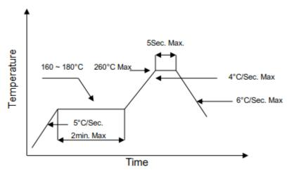
Note: Reflow soldering can be operated only one time. During the temperature ramp-up, no forces may be exerted on the diode which could
