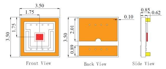
VD-0850I-003W-3E-2A0 with Substrate 3=Cu/Ag and Package E=7060 (unit: mm)
