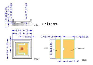
VD-0850I-001W-3E-2A0 with Substrate  $3=\underline{\text{Cu/Ag}}$  and Package  $E=\underline{7060}$  (unit: mm)
