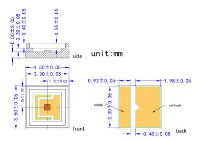
VD-0850C-200M-3E-2A0 with Substrate 3=Cu/Ag and Package E=7060 (unit: mm)
