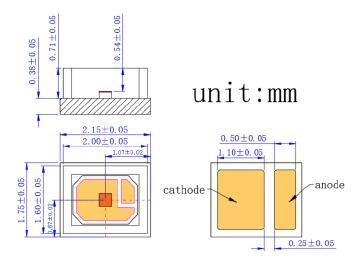
VD-0850C-200M-1C-2A0 with Substrate 1=AIN and Package C=3535 (unit: mm)
