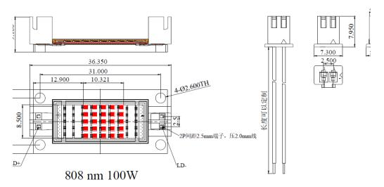
VD-0808I-100W-1U-2A0 + Water cooling with Substrate 1=<u>AIN</u> and Package U=<u>2511</u> (unit: mm)
