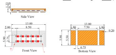
VD-0808I-025W-6K-2A0 with Substrate 6=<u>Cu</u> and Package K=<u>T-mount</u> (unit: mm)
