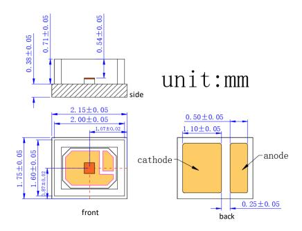
VD-0680C-005M-3A-2A0 with Substrate 3=<u>CuAg</u> and Package A=<u>2016</u> (unit: mm)
