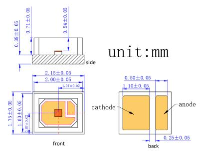
VD-0665C-003M-3A-2A0 with Substrate 3=CuAg and Package A=2016 (unit: mm)
