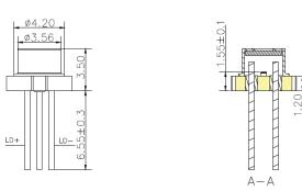
VD-0665C-003M-5I-2A0 with Substrate 5=<u>NiFe</u> and Package I=<u>TO46</u> (unit: mm)
