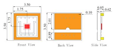
VD-0665C-003M-5H-2A0 with Substrate 5=<u>NiFe</u> and Package H=<u>TO56</u> (unit: mm)
