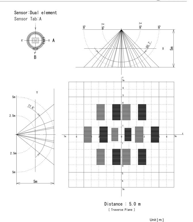
Measured with Nicera Standard 72.5dB amplifier when human body with 4 degrees C of temperature difference to environment moves at 1m/sec speed.
