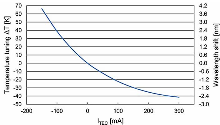
\* TEC performance is dependent on heat load, ambient temperature and heatsink properties
