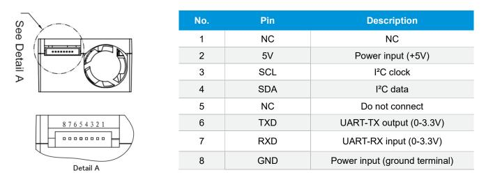
The interface connector is located at the side of the sensor.
