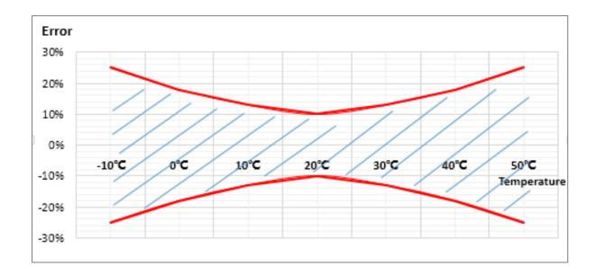
Particle measured error: under  $25\pm2^{\circ}$ C,  $50\pm10\%$ RH,  $0\sim1000\mu g/m^3$ , consistency and accuracy of PM1.0/PM2.5 is  $\pm10\%$  reading or  $\pm10\mu g/m^3$ , use the biggest one
