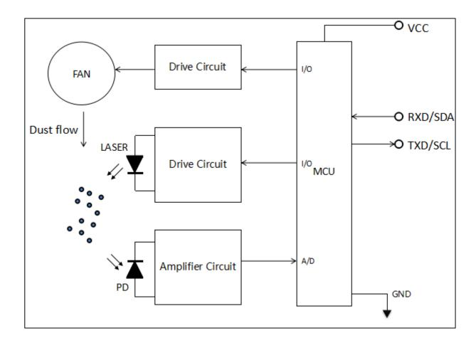
According to the above figure, The light source part of PM2012 is composed of a laser tube and a driving circuit. The detection part of the sensor is composed of light sensitive part which receives reflected light and amplifying circuit. Data processing and communication output are completed by microprocessor.
