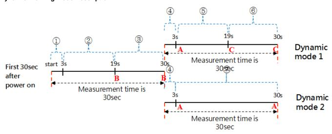
After sensors are in dynamic working mode, start measuring every 30s. The sensor starts the measurement for the first 3 seconds.
