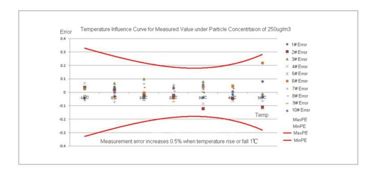
Particle measured error: under  $25\pm2\,^{\circ}$ C,  $0\sim1,000~\mu g/m^3$ , consistency and accuracy of PM1.0/PM2.5 is either  $\pm15\%$  reading or  $\pm15\mu g/m^3$ , the bigger one is considered.
