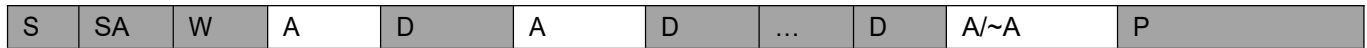
Picture 2: The general data format sends from the master device to the slave
