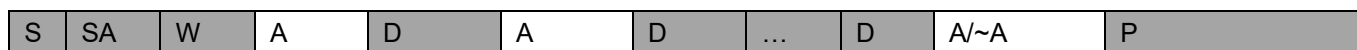
Picture 2: The general data format sends from the master device to the slave
