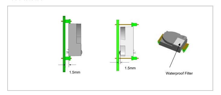
2. To avoid the influence of stress on sensor, please soldering by hand as much as possible when mounting the sensor to the PCB.
