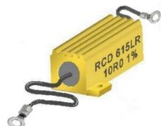
**Opt. L** (605-625): Insulated stranded wires embedded into the case. Black TFE 18AWG x 12" with 1/4" strip is standard (16AWG TFE & 14AWG PVC available). Also available with 4 insulated lead wires (**Opt. 4L**), and with a wide variety of terminals.
