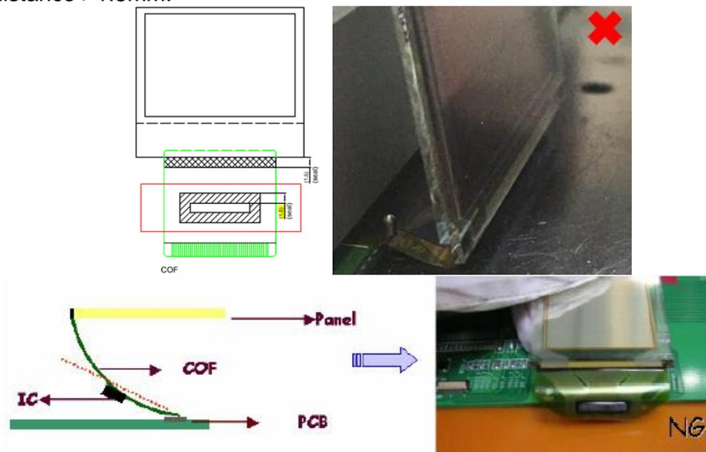
Use finger to insert COF /FPC into the connector when assembling the panel.
