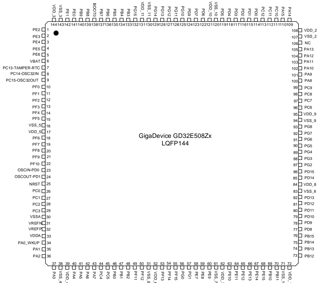
Figure 2-2. GD32E508Zx LQFP144 pinouts
