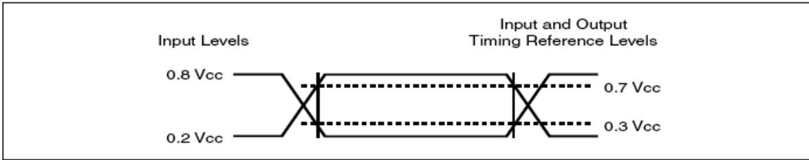
AC Measurement I/O Waveform
