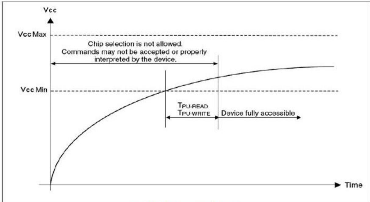
**Figure 31. Power-up Timing**
