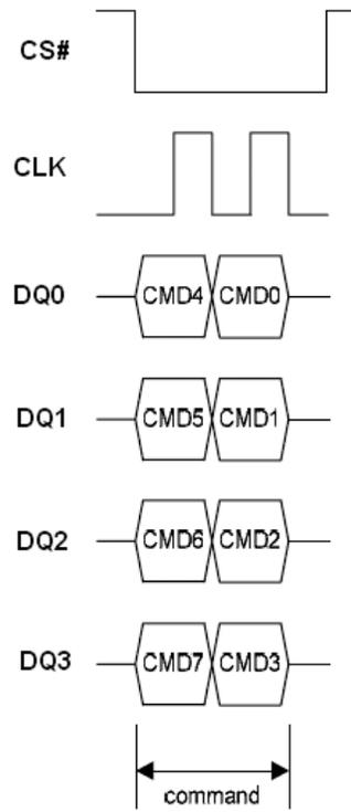
**Figure 29.1 Enter OTP mode Sequence in QPI Mode**
