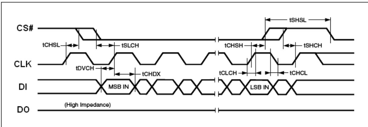
**Figure 34. Input Timing**
