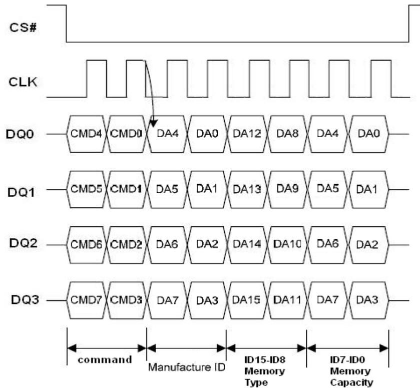
**Figure 28.1 Read Identification (RDID) in QPI Mode**
