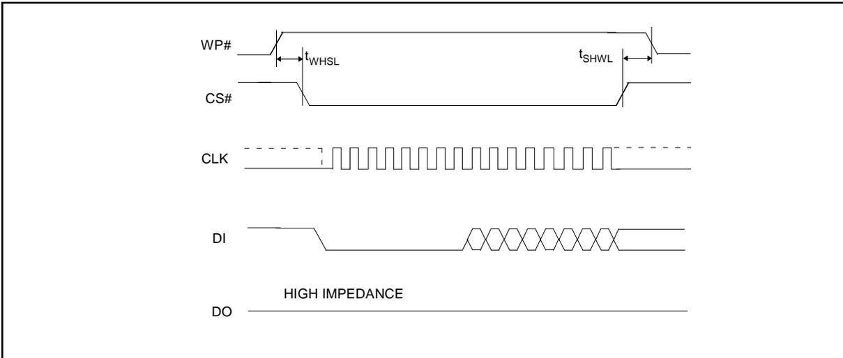
**Figure 36. Write Protect setup and hold timing during WRSR when SRP = 1**
