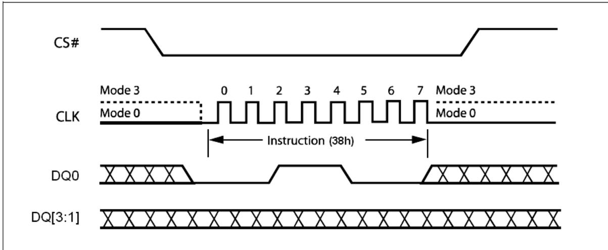
**Figure 6. Enable Quad Peripheral Interface mode Sequence Diagram**
