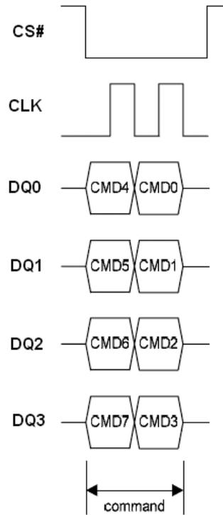
**Figure 23.1 Chip Erase Sequence in QPI Mode**
