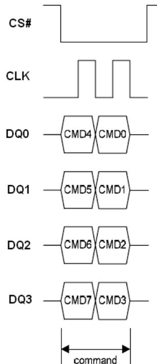
**Figure 9.1 Write Enable/Disable Instruction Sequence in QPI Mode**
