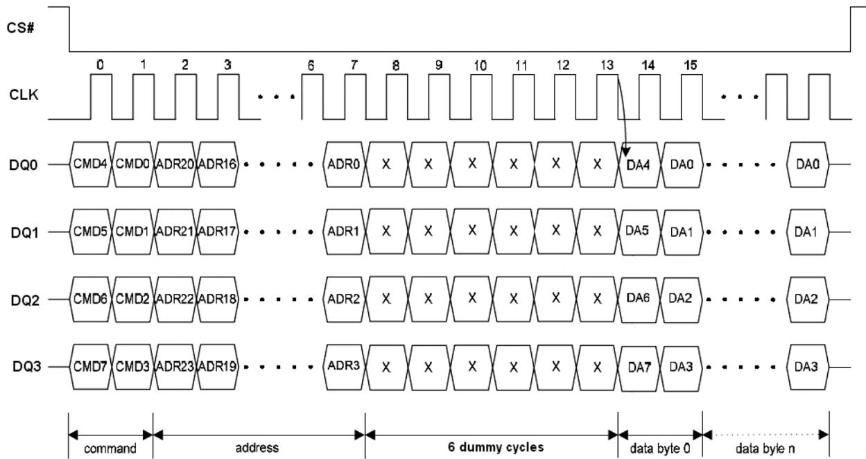
**Figure 13.1 Fast Read Instruction Sequence in QPI Mode**
