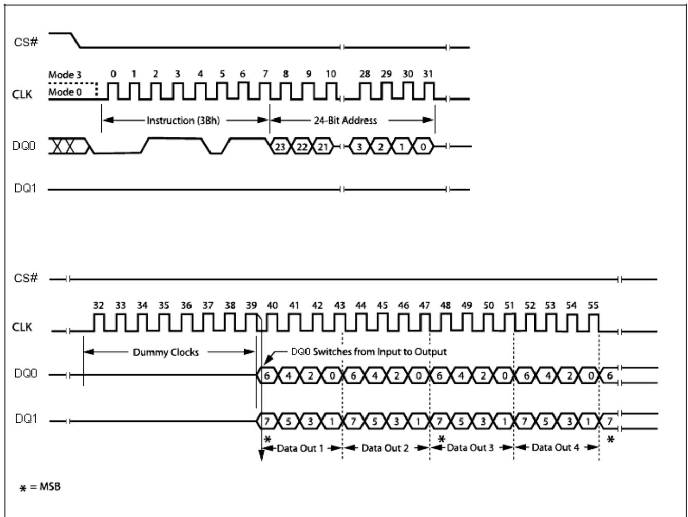
**Figure 14. Dual Output Fast Read Instruction Sequence Diagram**
