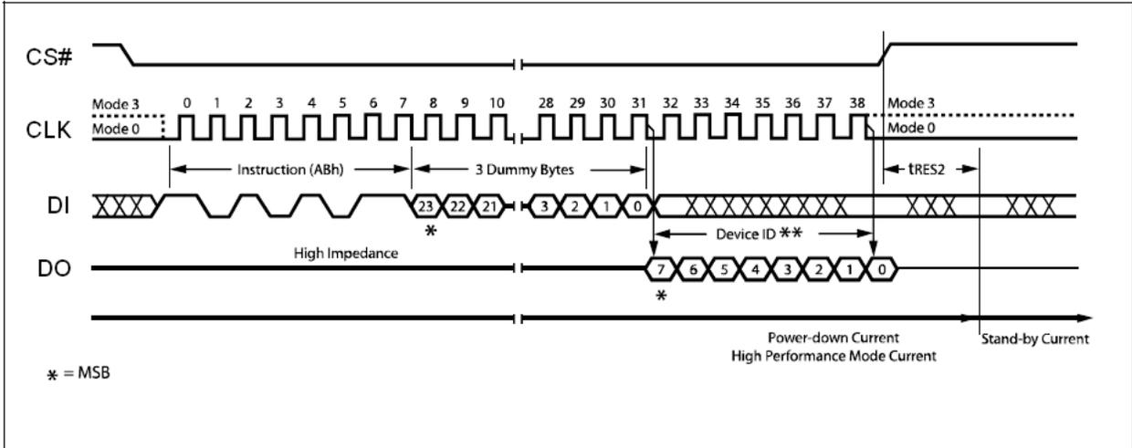
**Figure 26. Release Power-down / Device ID Instruction Sequence Diagram**
